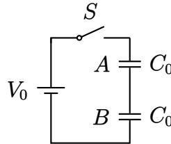
**Solution** While charging the capacitors, with the switch closed, we combine the two identical series capacitors into a single equivalent capacitor,
