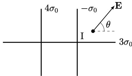
**Solution** The  $y$ -component of the electric field is solely due to the horizontal  $3\sigma_0$  plane. As this plane is positively charged, its electric field is directed away from itself, and therefore points upward in Region I,
