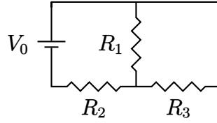
**Solution** We use the tabular method. Resistors  $R_1$  and  $R_3$  are in parallel, so we replace them with resistor  $R_4$ . Then, resistors  $R_2$  and  $R_4$  are in series, so we replace them with resistor  $R_5$ .
