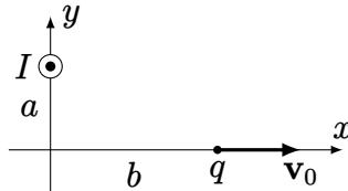
**Solution** Using the right-hand rule, the magnetic field circulates counter-clockwise about  $I$ ,
