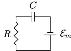
This is our basic  $RC$  charging circuit. Initially, when the capacitor is uncharged, the potential difference across resistor  $R$  is equal to  $\mathcal{E}_m$ . Using Ohm's law, the initial current is  $I_0 = \mathcal{E}_m / R$ . As the capacitor charges, the current through the circuit decays with time constant  $\tau = RC$ ,
