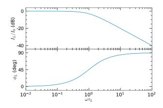
Shown above is the circuit's frequency response. At very low frequencies,  $\omega \tau_L \ll 1$ , the inductor acts as a dead short, and the current through the inductor is the same as the source's current. At higher frequencies, it begins to get harder to drive current through the inductor. We say that the inductor's current rolls off at frequency  $\omega = 1/\tau_L$ .
