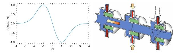
As the toroid's current is *increasing*, for t < 0, current is induced on the straight wire in the  $\hat{\mathbf{z}}$  direction to oppose this change. After the pulse's peak, the toroid's current is *decreasing*, and current is induced on the straight wire in the  $-\hat{\mathbf{z}}$  direction. The induced current's peak magnitude occurs at  $t = \pm \tau$ .
