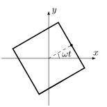
**Solution.** The loop's rotation is irrelevant in applying Faraday's flux rule, as the net flux through the loop does not depend on the loop's angle-of-rotation. The net emf is due to the electric field induced by the time-varying magnetic field. This, however, does not mean that the motional emf is zero throughout the loop. There are portions of the loop having a nonzero motional emf, but the net motional emf along each side sums to zero.
